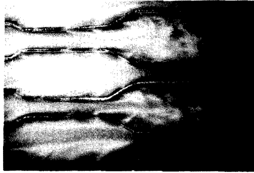
Fig. 3. Aspect of water flow in advanced heat exchanger ( Re = 400 ).
